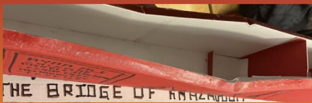
Bridge post failure. Top deck failed along the glue
