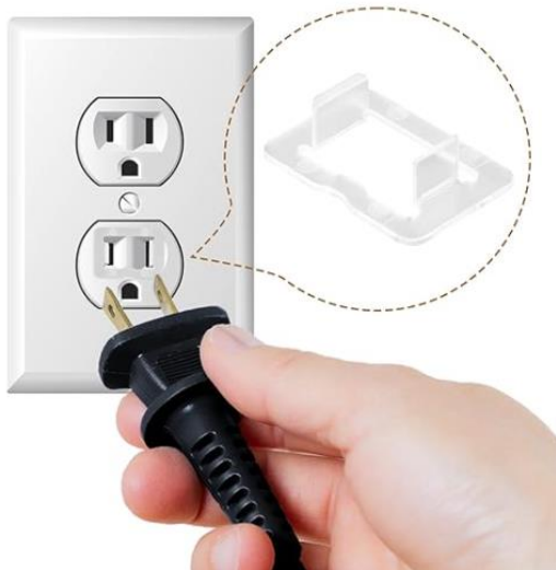
Figure 6: Above is a generic version of the plastic insert that can be placed into a wall socket thereby effectively reducing the size of the opening and increasing the friction of the pins in the wall socket [18].
